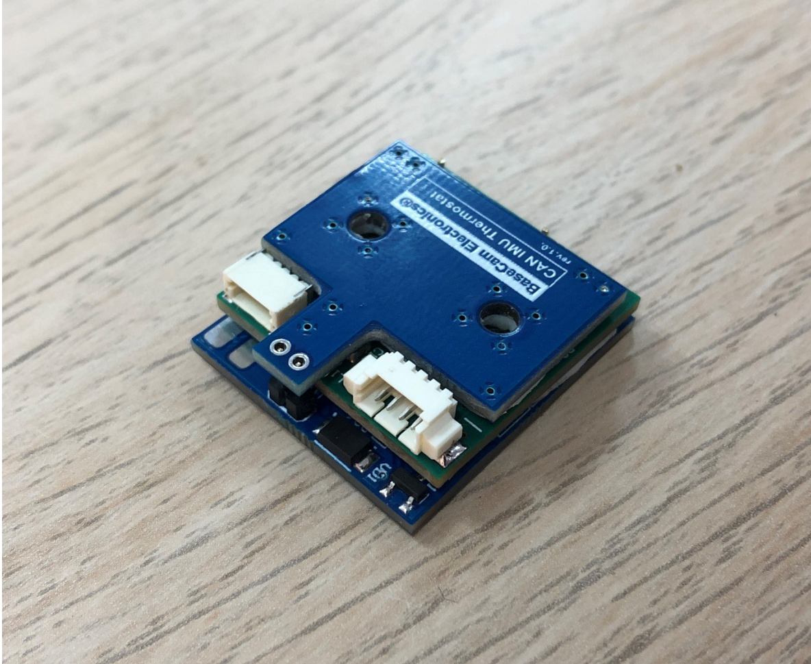
Figure 6. Installing the top thermostat board
